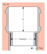
To establish pipe length required, loosely insert socket and follow Step 6 in Fixed Socket Section.
