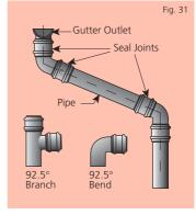
Also, any joint which is in the horizontal position such as 90°Branch arms or Bends etc.
